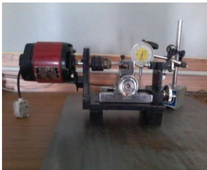
Fig 4 Alignment test on Machine bed
