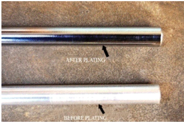
Fig. 1. Aluminium rod a) After Electroplating b) Before Electroplating.
