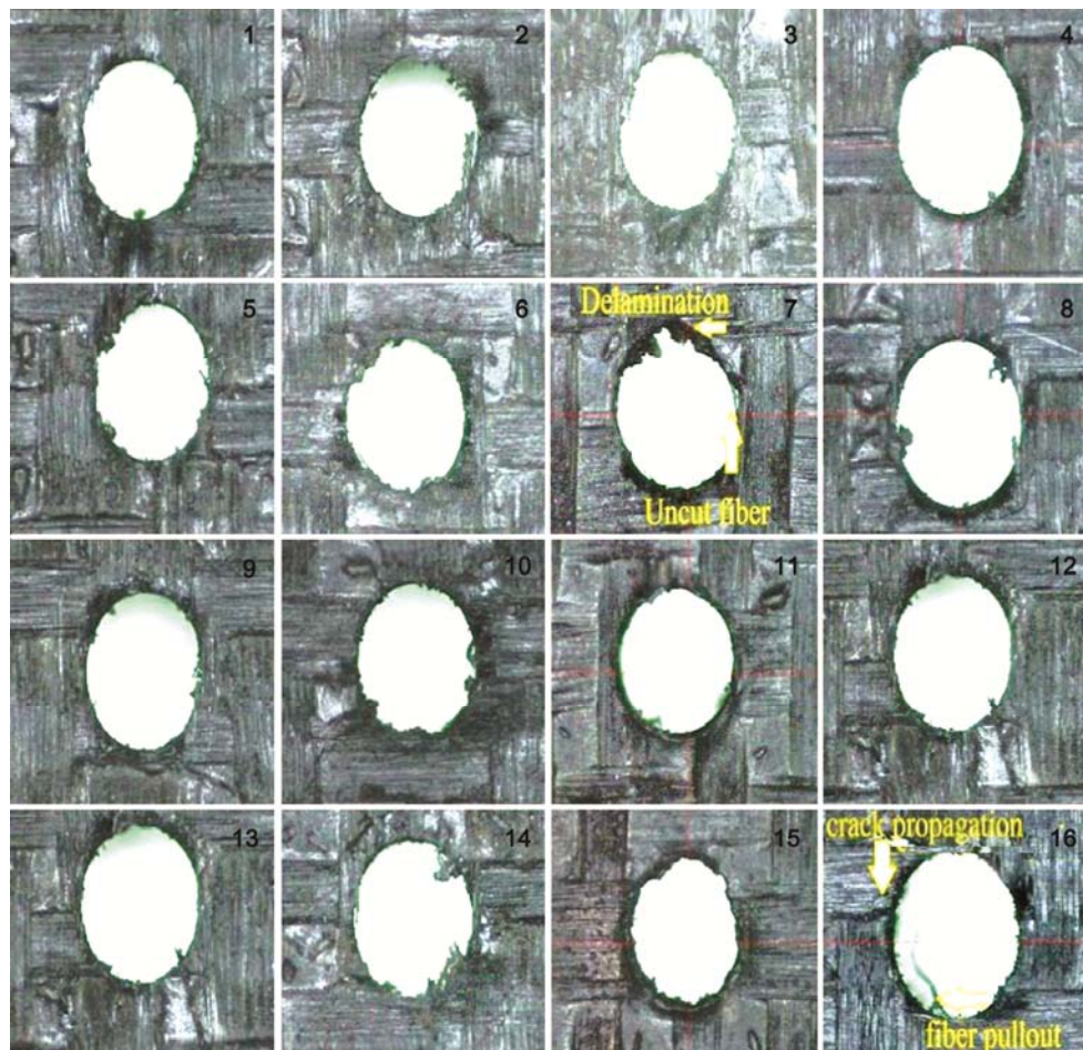
Fig. 8 — Machined hole at the entry side in MD.
