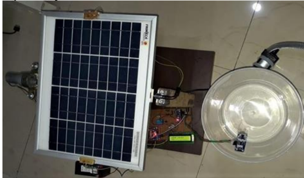
Figure 6:Solar Tracking and water pumping unit RFID-Technology:
