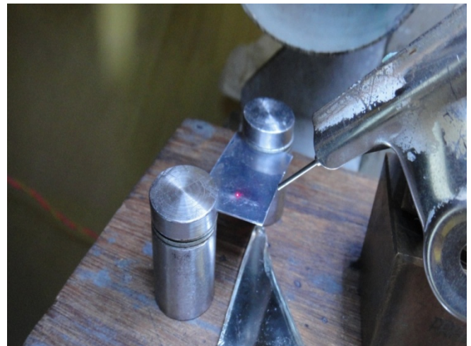
Figure: 6.2 Cutting stainless steel in ND: YAG laser machine
