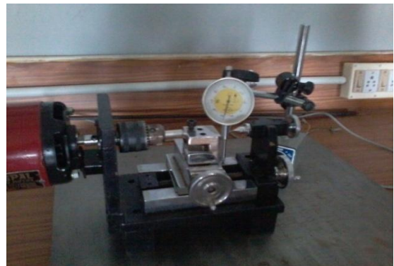
Fig.3 Alignment test on cross slide
