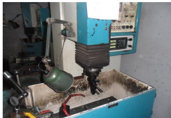
Figure 2 Spark EDM experimental setup
