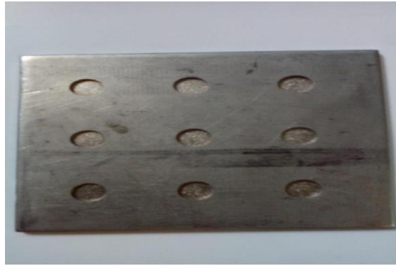
Figure 6 Work piece after drilling
