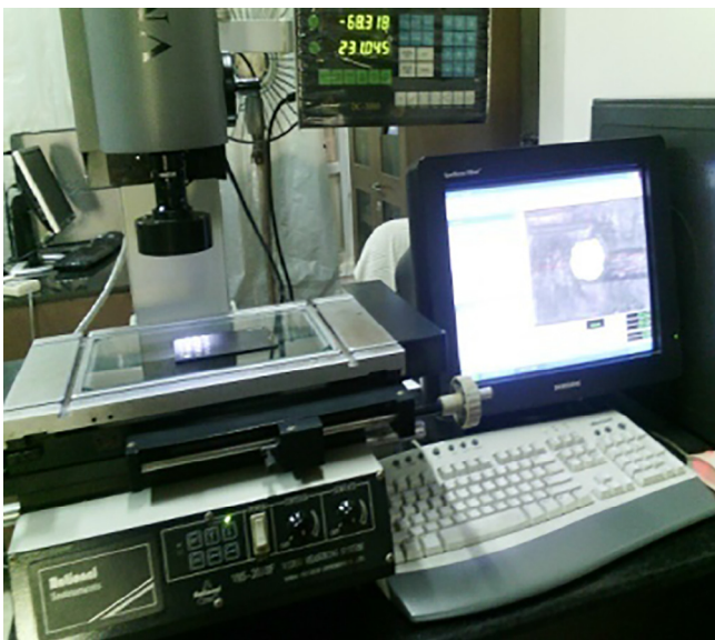
Fig. 2. Experimental setup of video measurement system.
