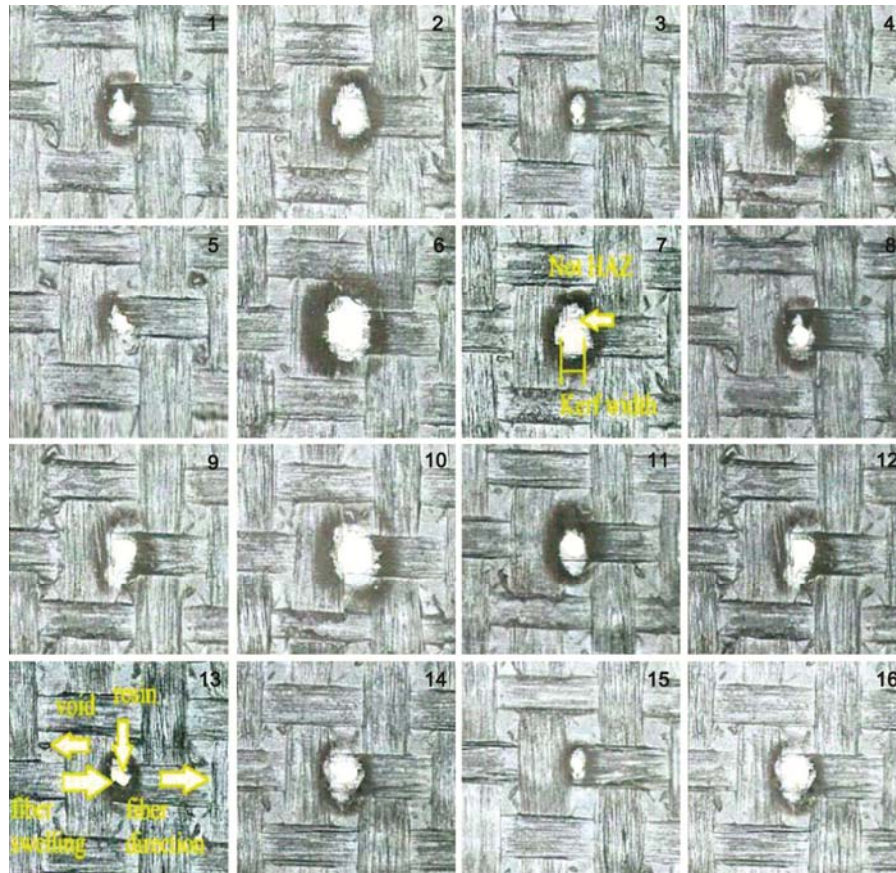
Fig. 11 — Machined hole at the exit side in LD.
