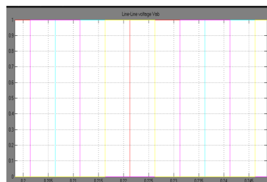
Fig 9. pulses of three phase inverter by an SPWM technique
